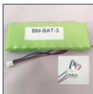
Rechargeable battery: Ni-MH (10 cell, 1line, 12V, 2200mA/h) Item Code: BM-BAT-3
