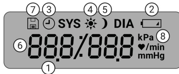
1. **Time** - Shown when the monitor is not taking a reading.
